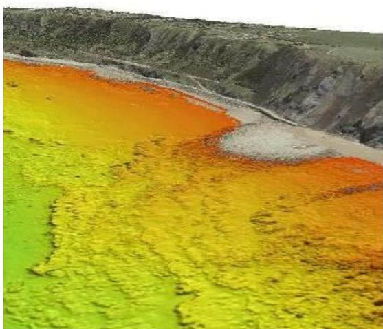
**Figure 6 3D imagery from integrated topographic, Lidar and bathymetric data**
